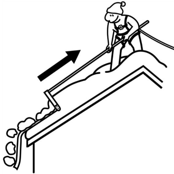
SnowPeeler is uniquely designed with a patent-pending, reversible frame adapter. This enables the user to effectively remove snow while working from the ground level or while positioned at the peak of the roof. With the rooftop configuration, the sectional pole is mounted on the top of the cutting frame in the opposite direction of the slide. With this application, the slide hangs over the edge of the roof and the cutting frame is pulled towards the user at the peak of the roof.
